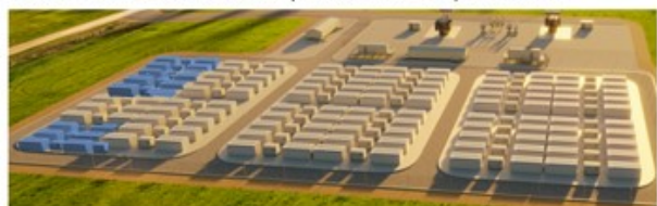
ILLUSTRATIVE VBB EXPANSION (300MW / ~520MWh) i.e. +70MWh
