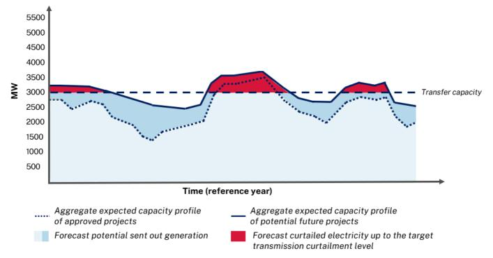
Figure 5: Headroom assessment - identifying the maximum available capacity profile
