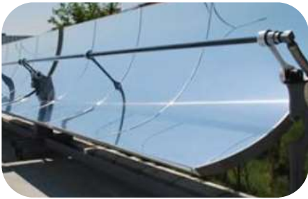
Parabolic trough: curved mirrors that reflect heat
