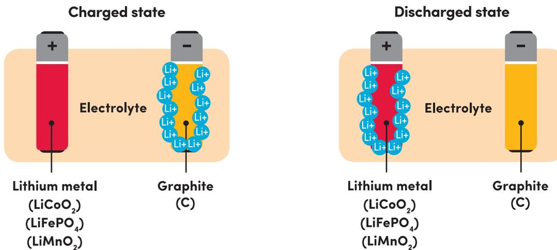
**Figure 20: Lithium-ion battery**
