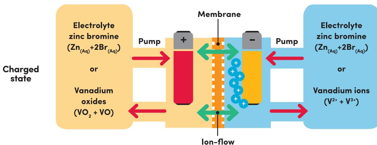
Figure 21: Flow battery
