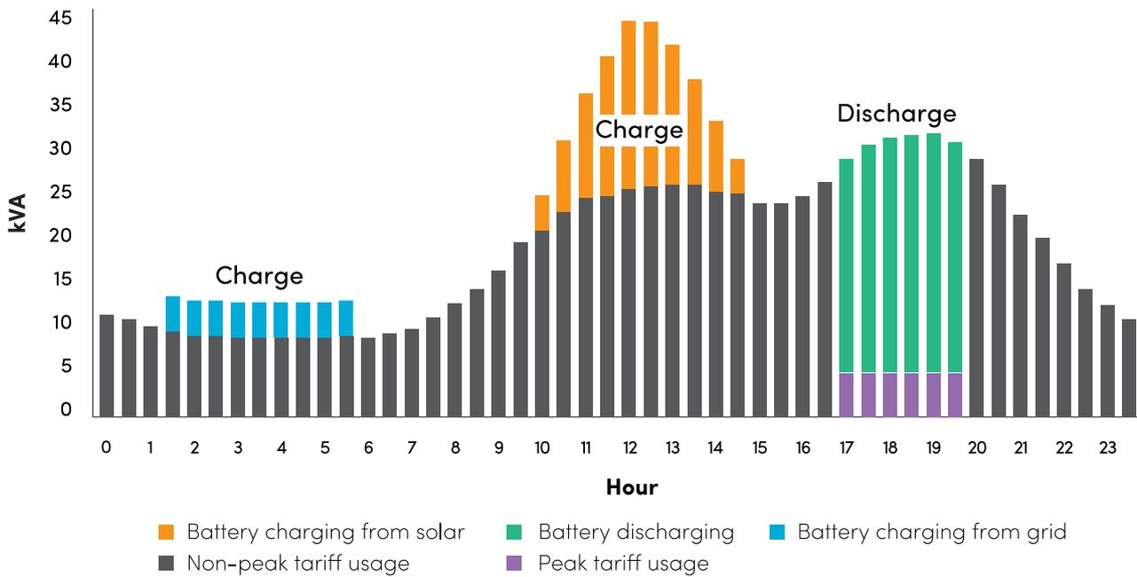
**Figure 11: Charging from both solar PV and from the grid off-peak/discharging in peak tariff period**
