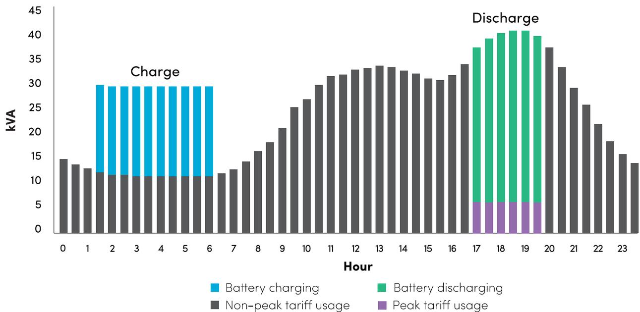
Figure 10: Charging from the grid off-peak/discharging in peak
