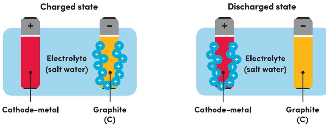
**Figure 22: Salt-water battery**
