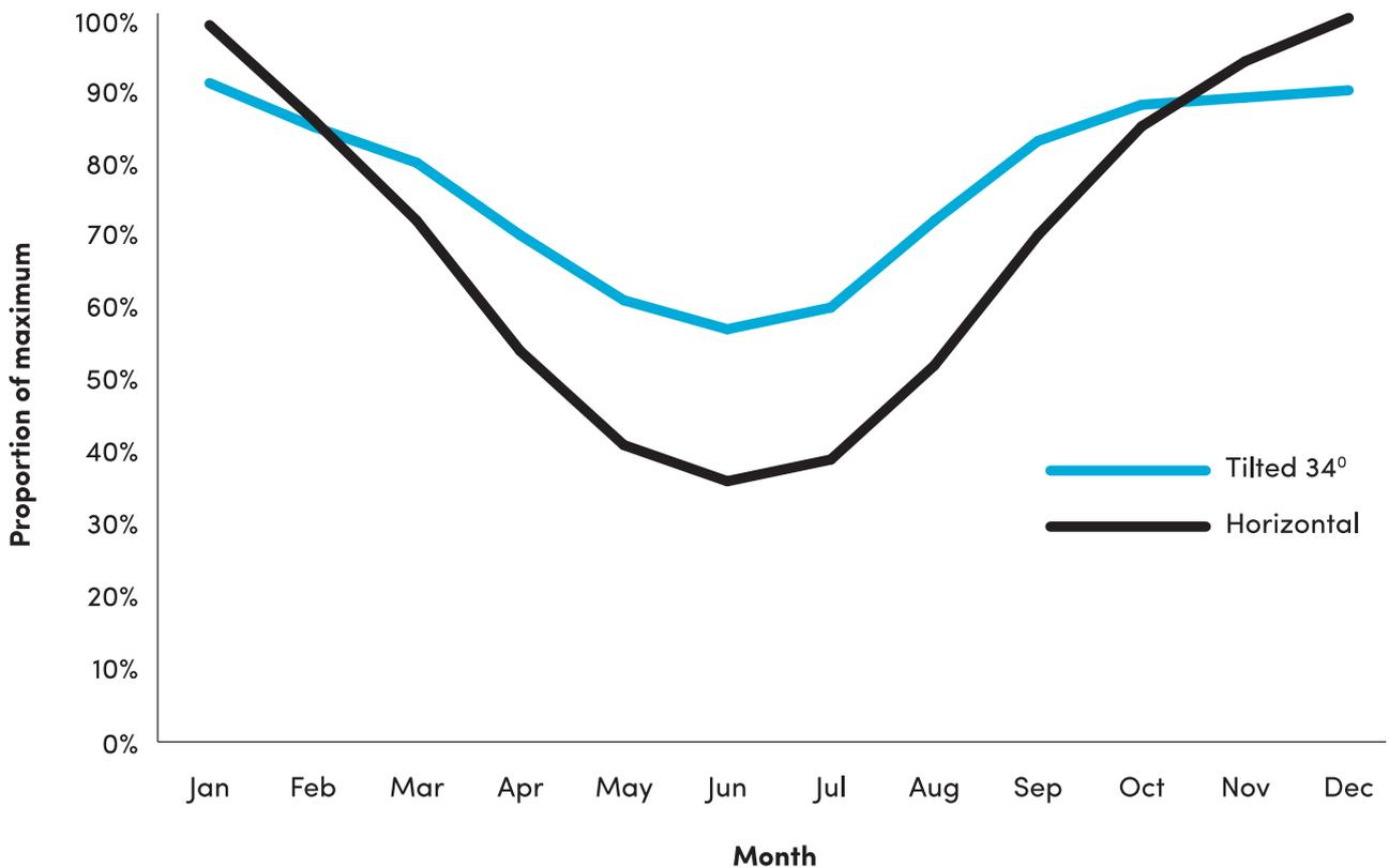
**Figure 15: Typical solar energy on a tilted vs horizontal panel (Sydney)**
