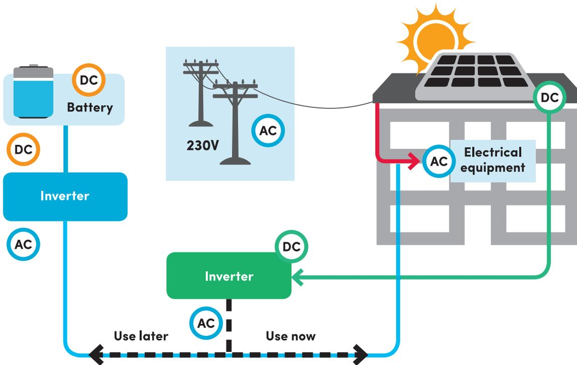
Figure 18: Grid connection with battery storage and solar PV
