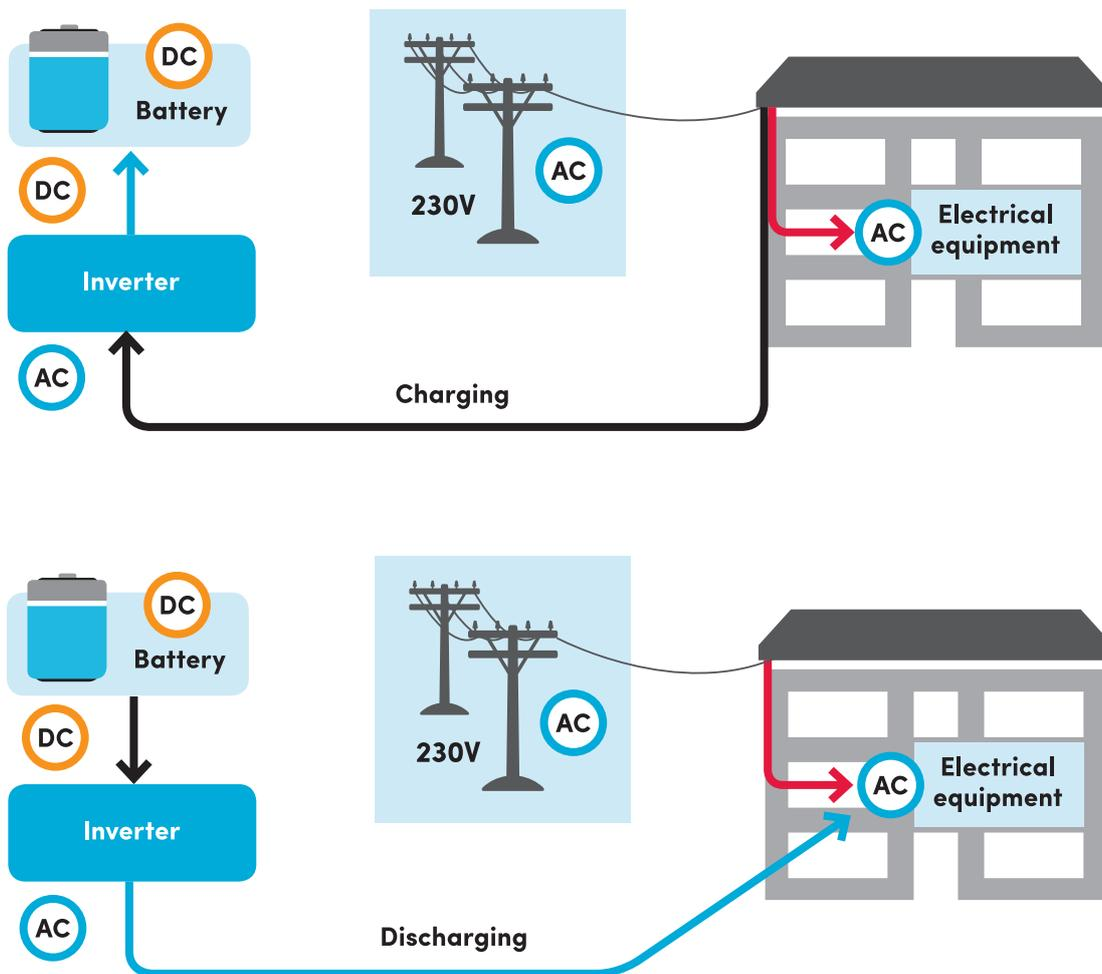
Figure 17: Grid connection with battery storage
