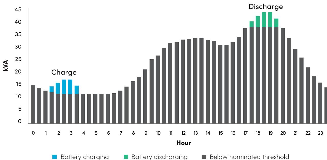
**Figure 12: Peak shaving to reduce capacity charges**
