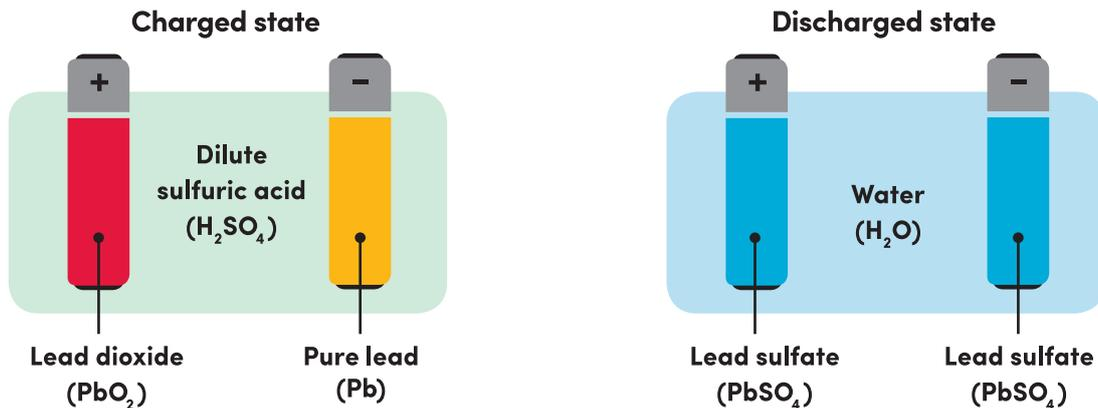
**Figure 19: Lead-acid battery**
