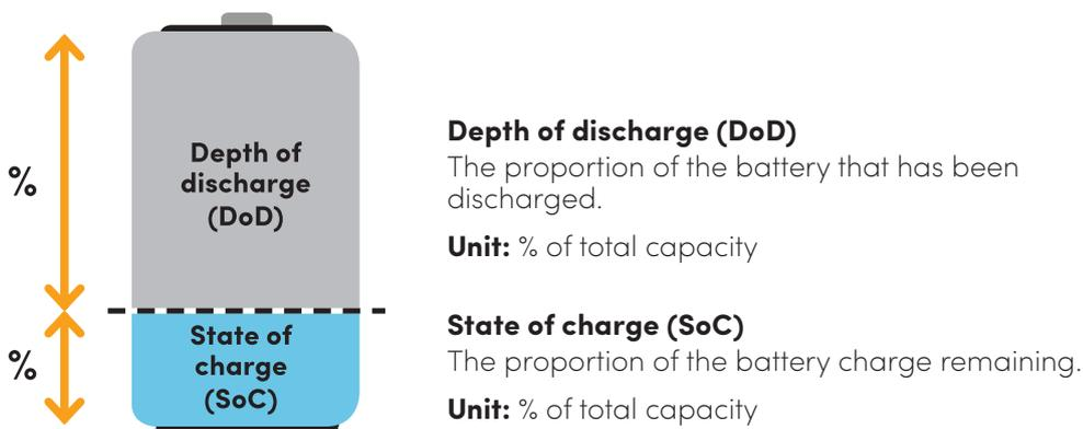
**Figure 7: State of charge and depth of discharge**
