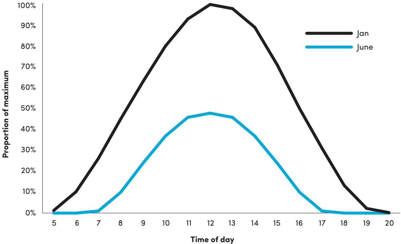
**Figure 14: Typical solar energy on a horizontal surface (Sydney)**
