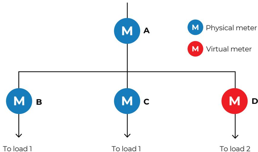
**Figure 11:** Single-line diagram noting physical and virtual meters
