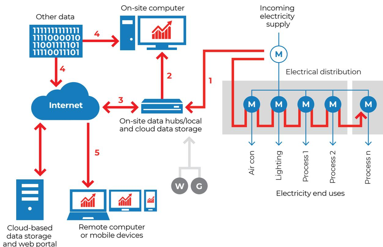
**Figure 8:** Typical components of an electricity metering and monitoring system
