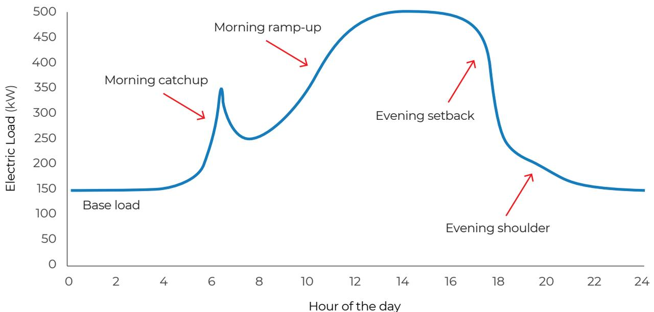
**Figure 14:** Stylised load shape for a typical office building in summer
