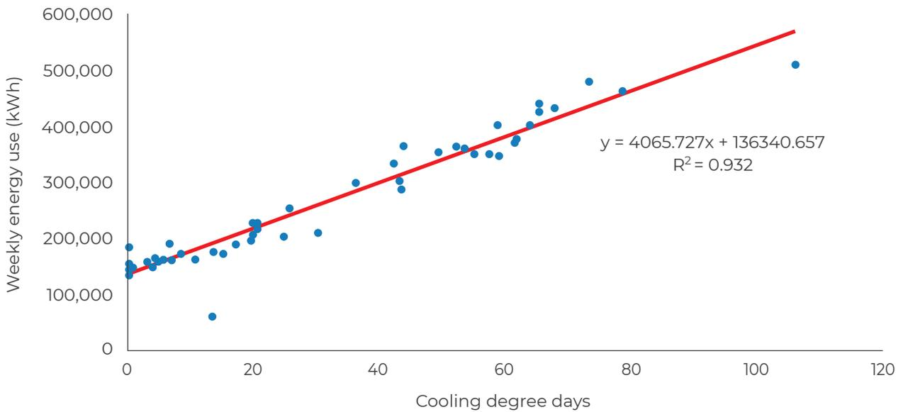
**Figure 17:** Example of regression analysis showing a correlation between temperature (expressed in cooling degree days) and energy use
