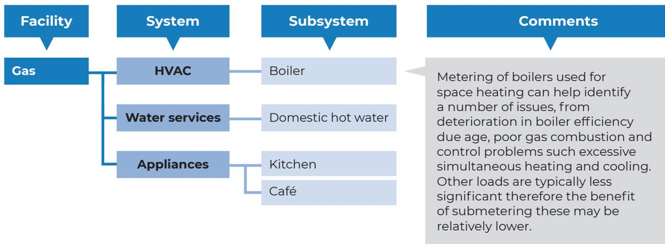
**Figure 16:** Example energy tree for a commercial building facility showing potential metering applications
