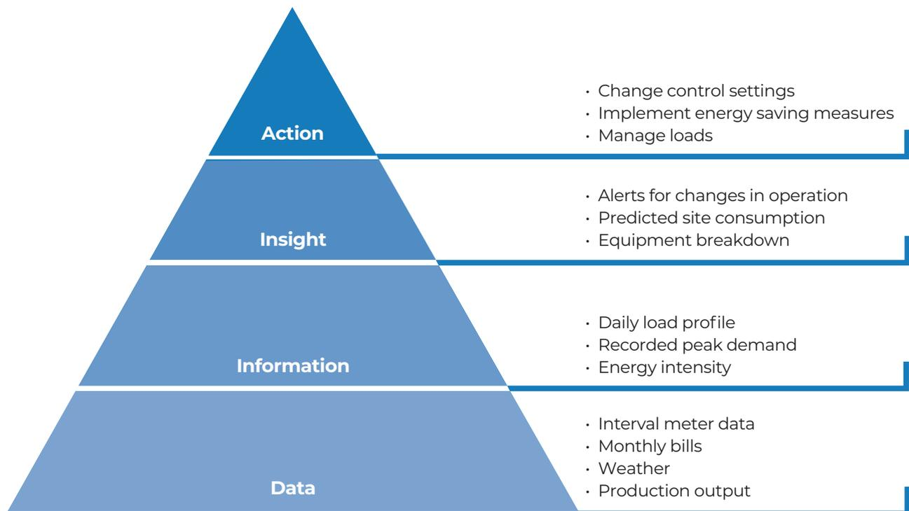
**Figure 7:** Hierarchy of information, from metering and monitoring to taking action
