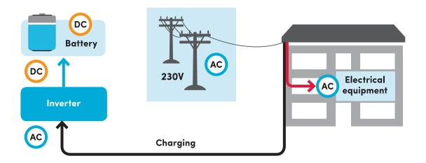
Figure 2: A battery system converts AC electricity, via an inverter, into DC electricity that charges a battery.
