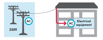
Figure 1: Electricity is generally supplied to businesses in New South Wales as alternating current (AC) at 230 volts single-phase or 400 volts three-phase.
