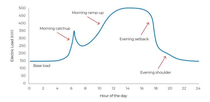
Figure 14: Stylised load shape for a typical office building in summer
