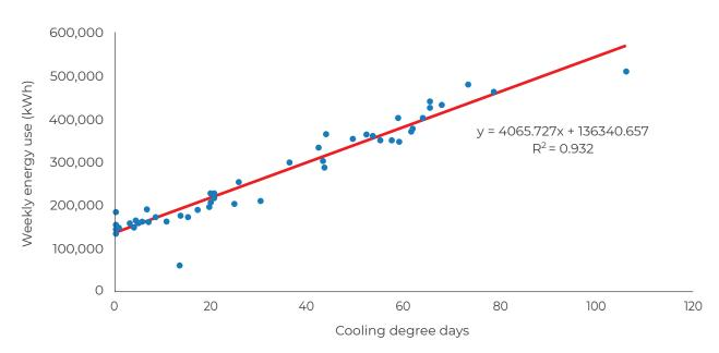
**Figure 17:** Example of regression analysis showing a correlation between temperature (expressed in cooling degree days) and energy use
