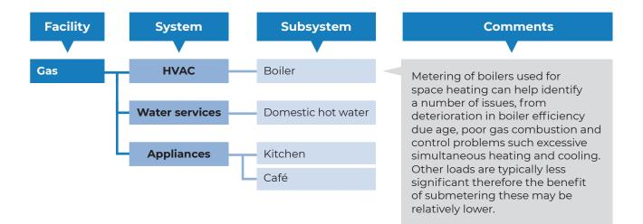
**Figure 16:** Example energy tree for a commercial building facility showing potential metering applications
