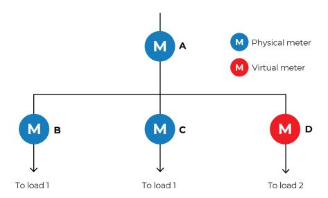
Figure 11: Single-line diagram noting physical and virtual meters
