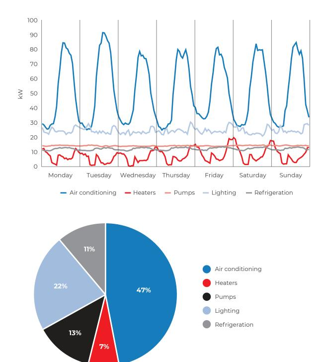
Figure 16: Equipment-level monitoring breakdown
