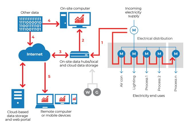
Figure 8: Typical components of an electricity metering and monitoring system
