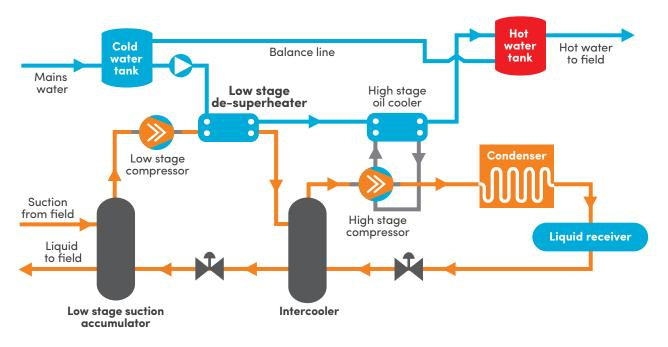
Figure 10: Schematic of heat recovery system with low-stage de-superheater
