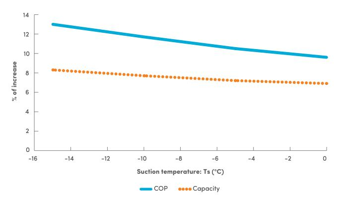
Figure 30: Coefficient of performance (COP) improvement due to removal of liquid injection oil cooling
