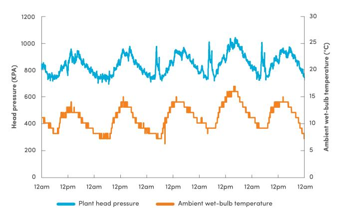
Figure 2: Typical plant head pressure under a variable head pressure control (VHPC) logic
