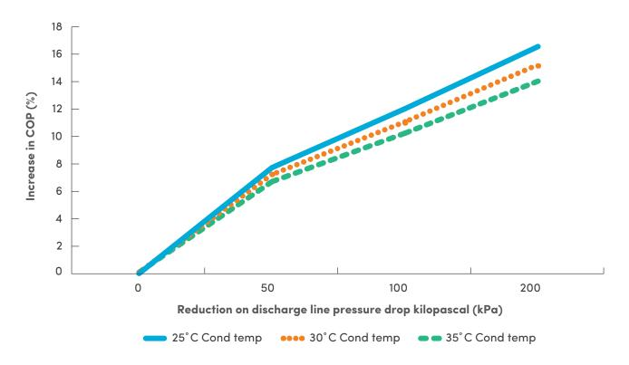
Figure 27: Effect of discharge pressure drop on the COP of a refrigeration plant
