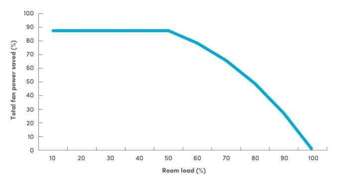
Figure 18: Fan power savings with room load
