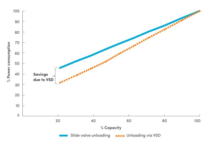
Figure 4: Slide valve and VSD control disparity
