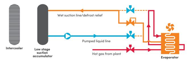
Figure 28: Schematic of conventional defrost relief technique
