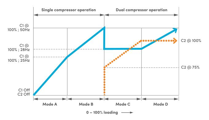
Figure 5: Example of efficient loading sequence on a two-compressor plant
