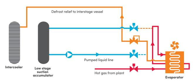
Figure 29: Schematic of energy efficient defrost relief technique
