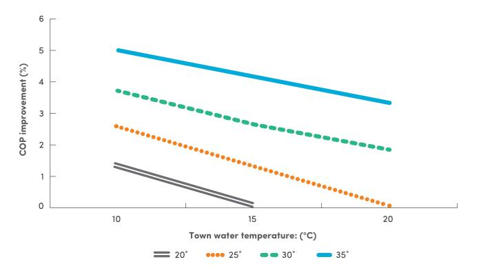
Figure 21: COP improvement due to condensate sub-cooling by town water
