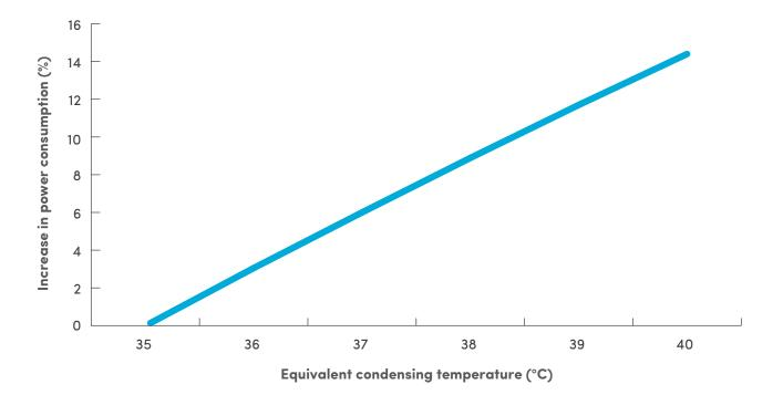
Figure 7: Effect of air in an ammonia refrigeration system
