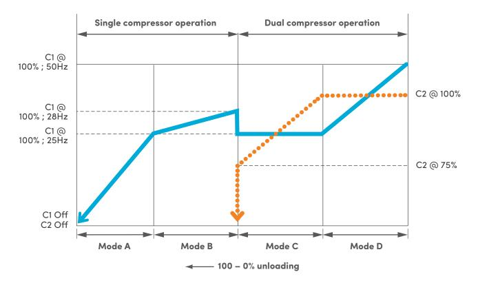
Figure 6: Example of efficient unloading sequence on a two-compressor plant
