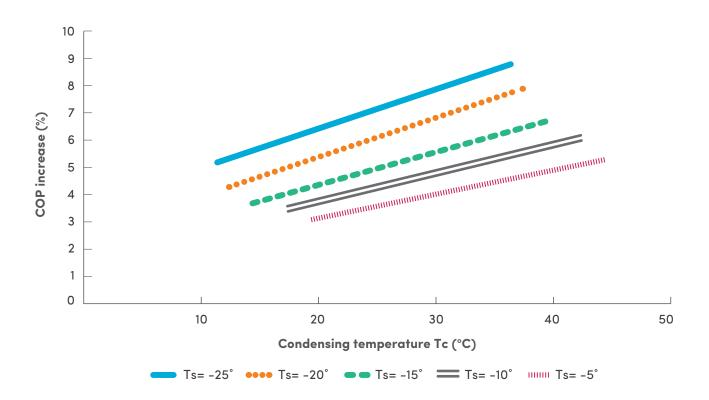
Figure 22: COP improvement due to condensate sub-cooling by high-stage economiser
