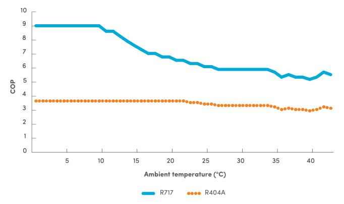
Figure B4: Effect of refrigerant choice on coefficient of performance (COP) of process chiller
