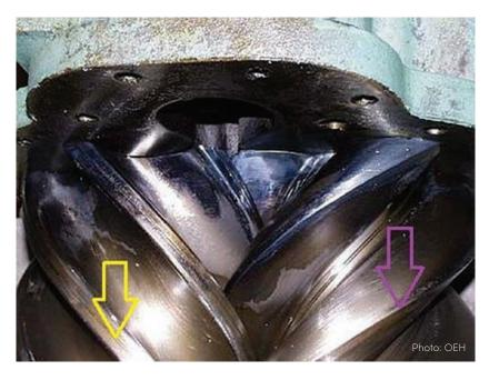
Figure 31: Screw compressor male (purple) and female (yellow) rotors with small ridges
