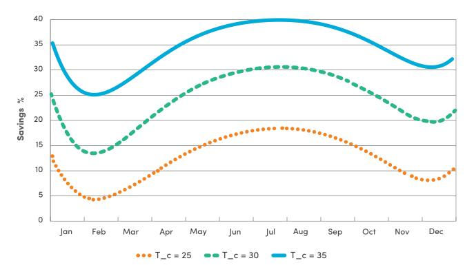
Figure B1: Annual energy saving profile due to variable head pressure control for a typical cold store application
