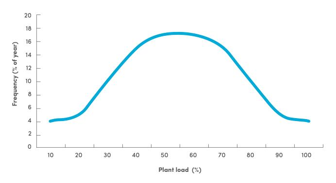
Figure 1: Refrigeration plant annual usage profile used for energy savings calculations
