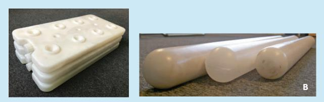
Figure 15: phase change materials (PCM) encapsulated in sealed rectangular (A) and tube (B) containers
